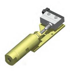
Pressure switch is electro hydraulic component with the task to send information about the achieved in advance specified pressure in the hydraulic or lubrication installation. Because of very precisely piston treatment and very small gap between piston and housing of few  $\mu$ m, any seal is not necessary.
