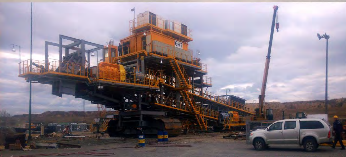
Mounting of central system for lubrication of reloading machine for surface mine „Gracanica“ Gacko, REPUBLIKA SRPSKA-Bosnia and Herzegovina
