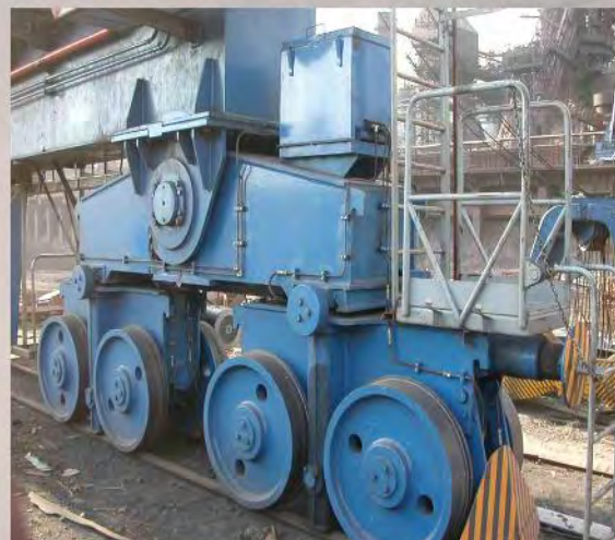
Part of the installation for lubrication of excavator's undercarriage for surface mine „Gracanica“ Gacko, REPUBLIKA SRPSKA-Bosnia and Herzegovina
