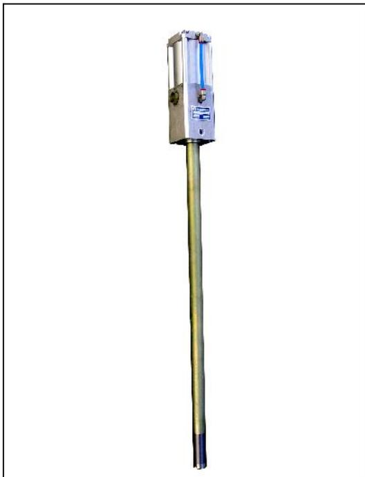
Pneumatic pump for oil draft is applied for oil draft for the barrels or tanks in service work-shops as well as in outdoor, where the supply of pressurized air is available. It is suitable for operation in very hard working conditions (excavators for surface exploitation, iron plants, cement works). This piston pump is designed to be directly mounted to the hole 2".
