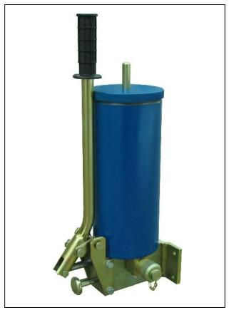
The hand pump 10-2450 used for small two-line lubrication systems. It is suitable for operation in very hard working conditions (excavators for surface exploitation, iron plants, cement works). This piston pump is equipped with tank, hand actuated distributing valve for line switching (R) and visual indicator with a weight.
