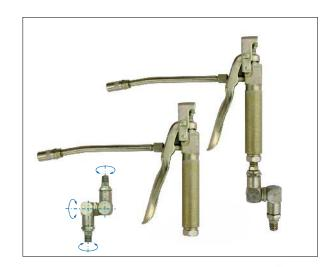
Lubrication gun is applied for single lubrication in industrial plants and service workshops. It is connected with electric or pneumatic driven power unit by highpressure hose. It is capable for operating in very hard conditions. Delivery can be with or without swivel joint. The swivel joint enable gun easily rotating around three axes. This makes the handling of the gun very comfortably despite of the rigidity of the high pressure hose. The hose of 350mm length is included in delivery
