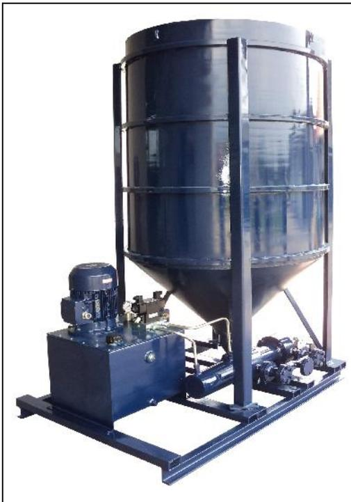
Electric driven pump for central supplement used in places there is a more grease lubrication central systems such as ironworks, rolling mills, coke plants etc. In this way is provided surely grease delivering to each pump by the pipelines. This ensures perfect grease purity. Also, the costs of lubricant handling are reduced because it's kept in one place. Head pumps can be automatically supplemented by installation of electric taps and control box.
