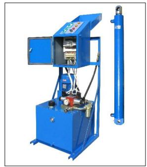
Actuator 90-0300 is applied oscillating motion with fixed amplitude according to the cylinder stroke. Movement of the cylinder rod can be continual or with a pause at the end position. Changing direction of the movement carried out without proximity switches so the device is insensitive of the dust and humidity.
