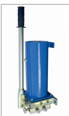
Hand pump operates in combination with double acting cylinder. High-pressure hose of 3 m length is included in delivery. Cylinder has to be ordered separately. Robust design, high precisely part treatment, high quality seals provide long time exploitation of the hand pump.
