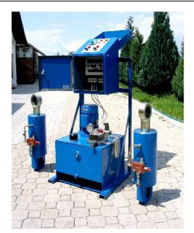
Actuator 90-0250 is applied for automatic correction of lateral deflection of the conveyors. The hydraulic cylinders swivel the band roller according to the signal from proximity detectors and keep the band in proper position. Control valve block assembled directly on the cylinder prevents the creep movements.
